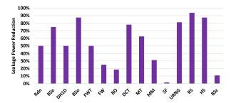
Figure 11. Estimated reduction in register file leakage power
