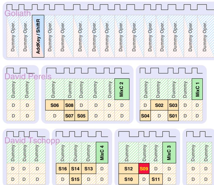
Figure 4.12: The operation is further randomized by changing the local clock generator period from cycle to cycle.
