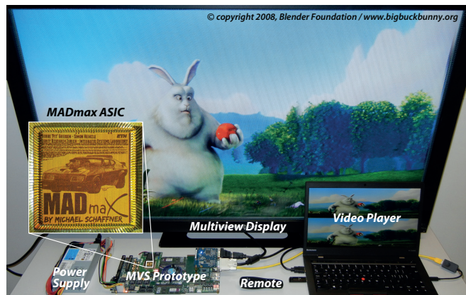
Fig. 1. Photograph of the running system. The MAD used in this setup is an Alioscopy HD 47 LV.
