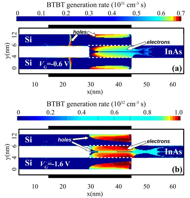
Fig. 9. Device (c): BTBT generation rate of an InAs-Si 2D-2D *p*TFET with  $T_{\text{InAs}} = T_{\text{Si}} = 4$  nm at (a)  $V_{\text{GS}} = -0.6$  V and (b)  $V_{\text{GS}} = -1.6$  V. The source-drain bias is  $V_{\text{DS}} = -0.5$  V.
