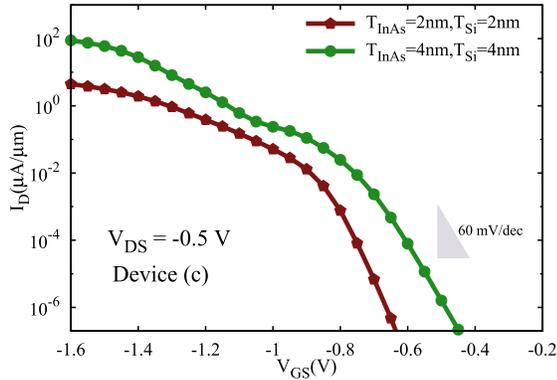
Fig. 8. Device (c): room-temperature  $I_{\text{D}}-V_{\text{GS}}$  characteristics of InAs-Si 2D-2D *p*TFETs at  $V_{\text{DS}} = -0.5$  V for  $T_{\text{InAs}} = T_{\text{Si}} = 2$  nm and  $T_{\text{InAs}} = T_{\text{Si}} = 4$  nm.
