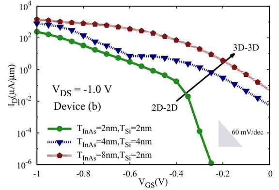
Fig. 6. Device (b): room-temperature  $I_D$ - $V_{GS}$  characteristics of InAs-Si 2D-2D pTFETs with  $V_{DS} = -1$  V.
