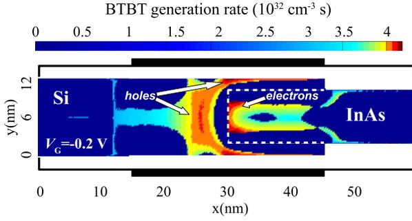
Fig. 7. Device (b): BTBT generation rate of an InAs-Si 2D-2D *p*-TFET with  $T_{\text{InAs}} = 8$  nm and  $T_{\text{Si}} = 2$  nm at  $V_{\text{GS}} = -0.2$  V and  $V_{\text{DS}} = -1$  V.
