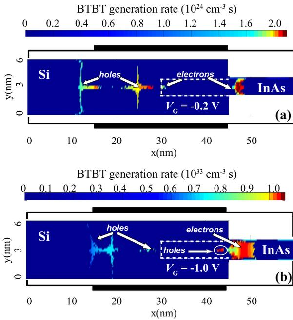
Fig. 5. Device (b): BTBT generation rate of an extremely thin InAs-Si 2D-2D pTFET with  $T_{InAs} = T_{Si} = 2$  nm at (a)  $V_{GS} = -0.2$  V and (b)  $V_{GS} = -1$  V. The source-drain bias is  $V_{DS} = -1$  V.
