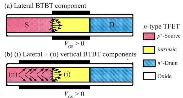
Fig. 1. Schematic of a double-gate n-type TFET exploiting (a) lateral BTBT, e.g., from source (S) to the intrinsic/drain (D) region, and (b) both lateral and vertical BTBT components. Notice that the vertical BTBT components occur under and almost perpendicular to the gate in the source.
