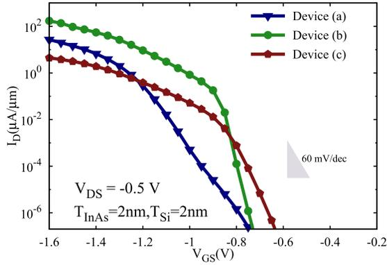
Fig. 4. Room-temperature  $I_D$ - $V_{GS}$  characteristics of InAs-Si 2D-2D pTFETs at  $V_{DS} = -0.5$  V for devices (a)-(c). The thicknesses are  $T_{InAs} = T_{Si} = 2$  nm in all cases.
