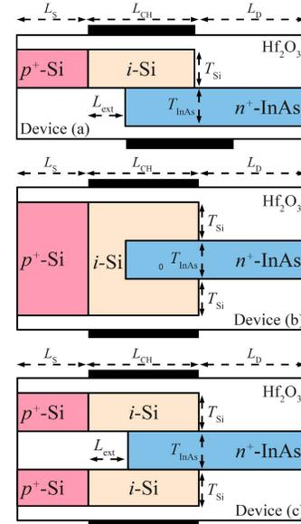
Fig. 3. Schematic of 2D–2D TFETs studied in this paper.  $L_S = 15$  nm,  $L_{CH} = 30$  nm, and  $L_D = 25$  nm. The oxide thickness under the gate region is  $T_{ox} = 1$  nm, whereas the doping concentrations for the source ( $n^+$ -type InAs region) and drain ( $p^+$ -type Si region) are  $N_D = N_A = 5 \times 10^{19}$  cm<sup>-3</sup>.  $L_{ext} = 15$  nm for devices (a) and (c). The temperature in the devices is assumed to be 300 K.
