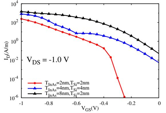
Fig. 2. Device (a): room-temperature  $I_D - V_{GS}$  characteristics of InAs-Si 2D-2D p-TFETs with  $V_{DS} = -1.0 \text{ V}$  computed with OMEN.
