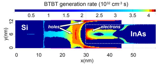
Fig. 3. Device (a): BTBT generation rate of an InAs-Si 2D-2D p-TFET with  $T_{InAs} = 8 \text{ nm}$  and  $T_{Si} = 2 \text{ nm}$  at  $V_{GS} = -0.2 \text{ V}$  and  $V_{DS} = -1.0 \text{ V}$ . Here, in a post-processing step, the potential from OMEN has been used as an input.
