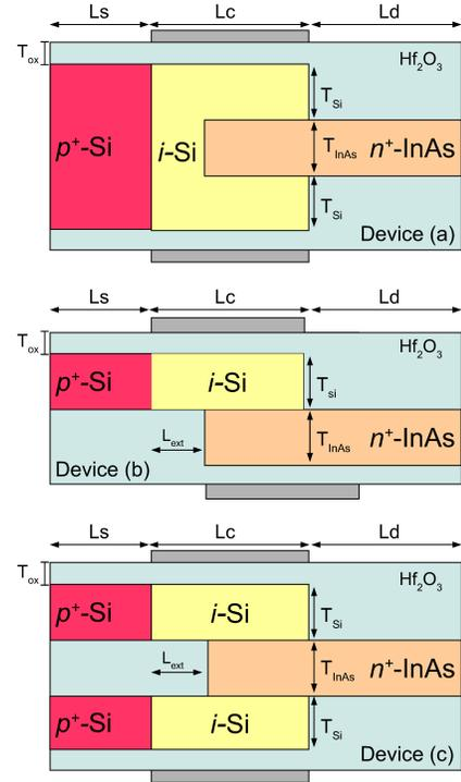
Fig. 1. Schematic view of the 2D-2D DOS switch TFETs studied in this work.  $L_s = 20$  nm,  $L_c = 30$  nm and  $L_d = 20$  nm. The oxide thickness under the gate region is  $T_{ox} = 1$  nm, whereas the doping concentrations for the source ( $n^+$ -type InAs region) and drain ( $p^+$ -type Si region) are  $N_D = N_A = 5 \times 10^{19}$  cm $^{-3}$ . For the devices (b) and (c)  $L_{ext} = 10$  nm. The temperature in the devices is assumed to be 300 K.
