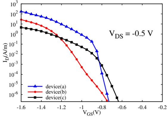
Fig. 4. Room-temperature  $I_D - V_{GS}$  characteristics of InAs-Si 2D-2D p-TFETs, at  $V_{DS} = -0.5$  V for devices (a) (triangles), (b) (dots) and (c) (squares), computed with OMEN. The thicknesses are  $T_{\text{InAs}} = T_{\text{Si}} = 2$  nm in all cases.
