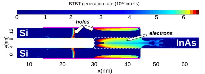
Fig. 6. Device (c): BTBT generation rate of a InAs-Si 2D-2D p-TFET with  $T_{\text{InAs}} = T_{\text{Si}} = 4$  nm at  $V_{GS} = -0.6$  V and  $V_{DS} = -0.5$  V. Here, in a post-processing step, the potential from OMEN has been used as an input.
