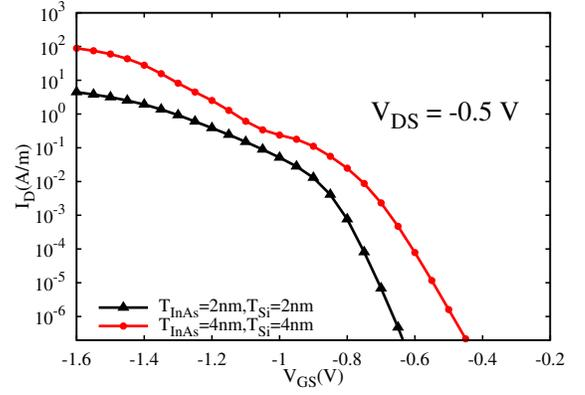
Fig. 5. Device (c): room-temperature  $I_D - V_{GS}$  characteristics of InAs-Si 2D-2D p-TFETs, at  $V_{DS} = -0.5$  V for  $T_{\text{InAs}} = T_{\text{Si}} = 2$  nm (triangles) and  $T_{\text{InAs}} = T_{\text{Si}} = 4$  nm (dots), computed with OMEN.
