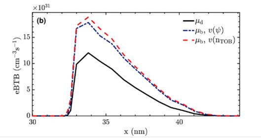
Fig.6: Electron BTBT rates for different electron mobilities ( $\mu_d = 1 \times 10^3 \text{ cm}^2/\text{Vs}$ ,  $\mu_b[v(\psi_n)]$ , and  $\mu_b[v(nTOB)]$ ) extracted at  $V_{GS} = 0 \text{ V}$  and  $V_{DS} = 2.5 \text{ V}$ .
