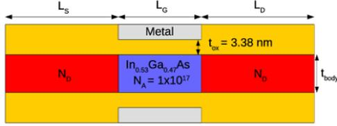
Fig.1: Schematic of an  $\text{In}_{0.53}\text{Ga}_{0.47}\text{As}$  double-gate (DG) ultra-thin-body FET. Parameters:  $N_D = 5 \times 10^{19} \text{ cm}^{-3}$ ,  $L_S = 20 \text{ nm}$ ,  $L_G = 11.5 \text{ nm}$ ,  $t_{\text{body}} = 4.2 \text{ nm}$ , and  $m_e = 0.0678 m_0$ .
