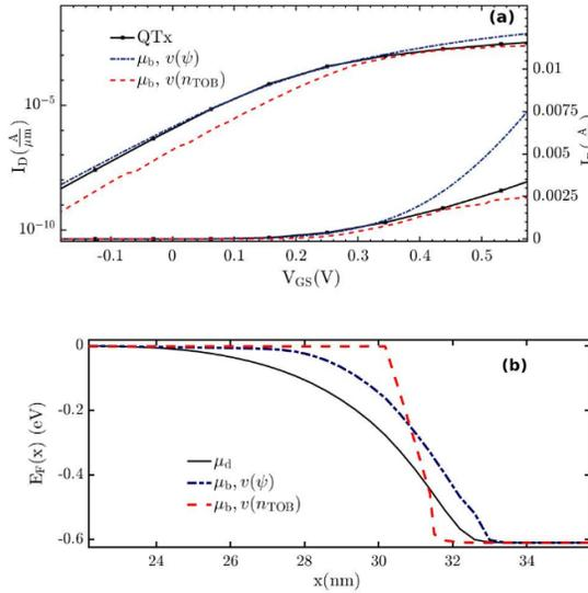
Fig.2: (a)  $I_D$ - $V_{GS}$  characteristics at  $V_{DS} = 0.61 \text{ V}$  of the device depicted in Fig. 1 with a tunnel mass  $m_t = m_e$ . (b) Fermi energy profiles  $-e\psi_n(x)$  for different electron mobilities ( $\mu_d = 1 \times 10^3 \text{ cm}^2/\text{Vs}$ ,  $\mu_b[v(\psi_n)]$ , and  $\mu_b[v(nTOB)]$ ), all extracted at  $V_{GS} = -0.2 \text{ V}$  and  $V_{DS} = 0.61 \text{ V}$ .
