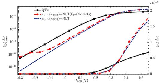
Fig.3:  $I_D$ - $V_{GS}$  characteristics at  $V_{DS} = 50 \text{ mV}$  of the device depicted in Fig. 1 with a tunnel mass  $m_t = m_e$ . The red curve was obtained by a post-processing calculation of the STDT current using the contact Fermi energies in the NLT model instead of local QFPs.
