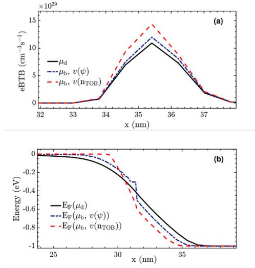
Fig.5: (a) Electron BTBT rates for different electron mobilities ( $\mu_d = 1 \times 10^3 \text{ cm}^2/\text{Vs}$ ,  $\mu_b[v(\psi_n)]$ , and  $\mu_b[v(nTOB)]$ ) extracted at  $V_{GS} = 0 \text{ V}$  and  $V_{DS} = 1 \text{ V}$ . Parameters are the same as in Fig. 4. (b) Corresponding profiles of the electron Fermi energy  $-e\psi_n(x)$ .
