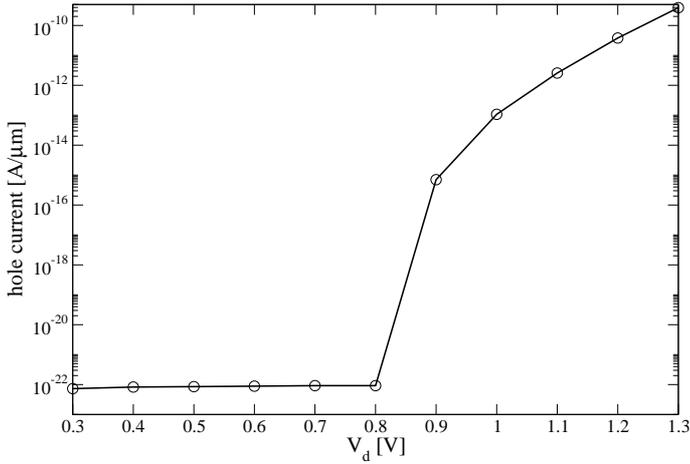
Figure 6: Hole current as function of drain voltage at  $V_g = 1.1V$ .
