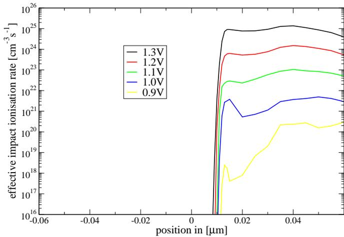
Figure 7: Profile of the effective impact ionisation rate as function of the drain voltage at  $V_g = 1.1V$ .
