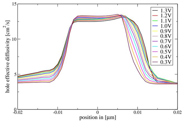
Figure 5: Profile of the xx-component of the hole effective diffusivity as function of the drain voltage at  $V_g = 1.1V$ .
