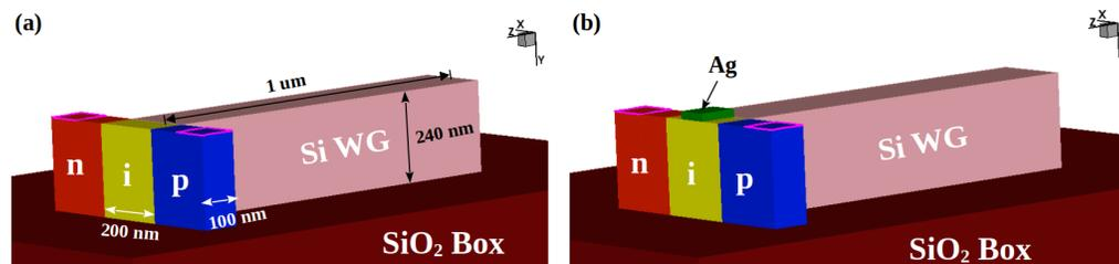
Figure 1. Sketch of studied device: (a) non-plasmonic and (b) plasmonic WGPD. The metal strip on the i-region of the plasmonic device is 80 nm/20 nm/100 nm long in x/y/z direction.
