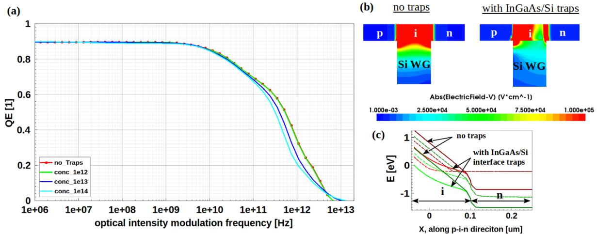
Figure 3. (a) Comparison of optical response curves obtained from an ideal and a defective non-plasmonic device with h-traps at the In<sub>0.53</sub>Ga<sub>0.47</sub>As/Si-WG interfaces having a concentration of 1e12, 1e13, and 1e14 cm<sup>-2</sup>eV<sup>-1</sup>. (b)/(c) Comparison of E-field profiles/band diagrams at -2V obtained from simulations without and with h-traps at the In<sub>0.53</sub>Ga<sub>0.47</sub>As/Si-WG interface with a concentration of 1e14 cm<sup>-2</sup>eV<sup>-1</sup>.
