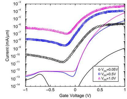
Fig. 9: Measured  $I_D V_{GS}$  characteristics [5] and simulated BTBT current assuming homogeneous 8% compressive in-plane strain. Gap extracted from Van de Walle model [16], effective masses from OMEN [7].
