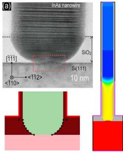
Fig. 4: TEM image of the InAs/Si nanowire TFET from Tomioka et al. [5] (upper left), simulation close-up (lower left), entire simulation domain with carrier concentrations (right).
