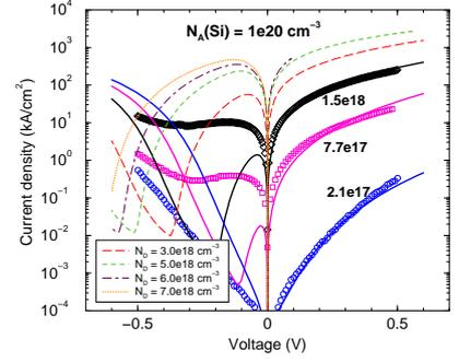
Fig. 3: Comparison between measured and TCAD-simulated InAs/Si nanowire hetero Esaki diodes. The ON-current is limited to  $\sim 1 \times 10^4$  kA/cm<sup>2</sup>, in good agreement with the homo diodes of Fig. 1.
