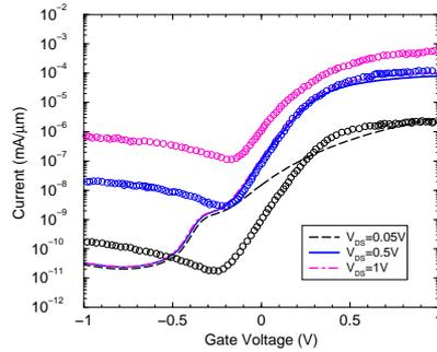
Fig. 8: Simulation with bulk DAT in restricted region (BTBT turned off). DAT parameters: zero-field lifetimes  $\tau_n = \tau_p = 3 \times 10^{-8}$  s, lattice relaxation energy  $S\hbar\omega_0 = 10.5$  meV, tunnel masses  $m_n = 0.023 m_0$ ,  $m_h = 0.2 m_0$ .
