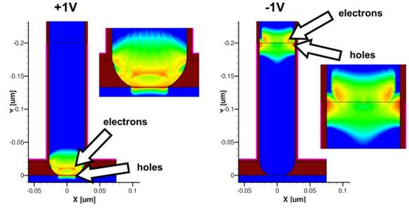
Fig. 6: BTBT rate distribution at  $V_{GS} = 1$  V (left) and  $V_{GS} = -1$  V (right). The strong ambipolar current is caused by off-junction tunneling under the gate edge which is aligned with the high-low doping transition. It can be suppressed by a corresponding gate “underlap”. The simulated ON-current at  $V_{GS} = 1$  V originates from in-junction BTBT with delta-like hole generation at the interface.
