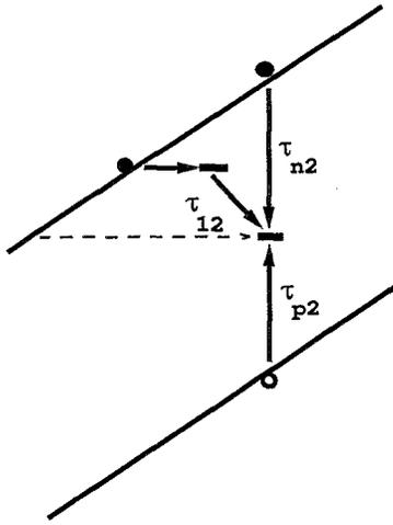
FIG. 3. Direct tunneling into the shallow donor-like state as a possible source of excess current. Tunneling into the midgap level is negligible because of the huge potential barrier. If  $\tau_{12} \ll \tau_{n2}$ , recombination via the upper level can become dominant, depending on its binding energy.
