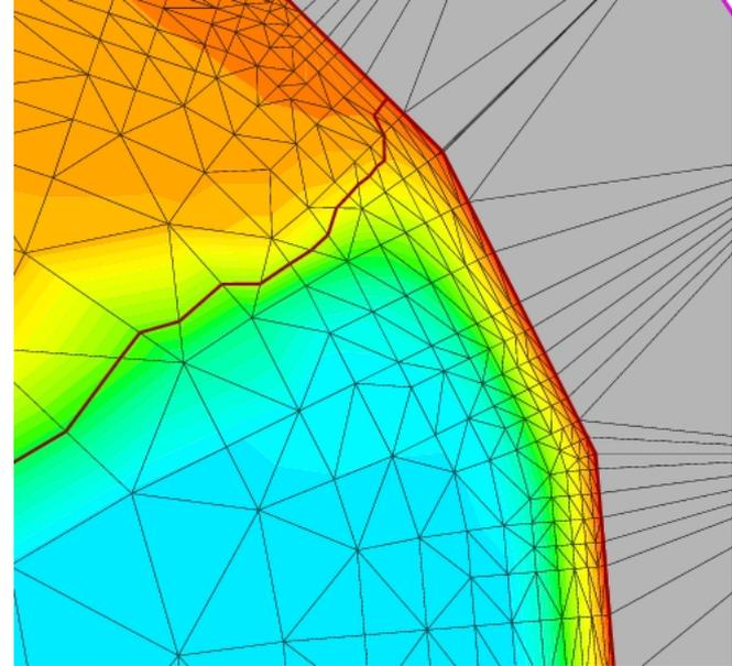
Quad-tree and normal-offsetting mesh with current density.
