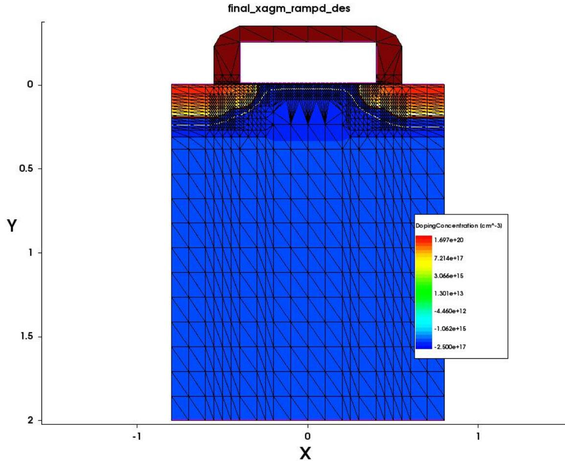
Schematic MOSFET model with underlying grid.
