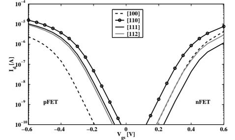
Fig. 3. FB transfer characteristics for  $L_g = 13 \text{ nm}$ . Left:  $I_d - V_{gs}$  ( $V_{ds} = -0.4 \text{ V}$ ) of p-FETs with transport directions along [100] (dashed line), [110] (solid line with circles), [111] (black line), and [112] (gray line). Right: n-FET curves for  $V_{ds} = 0.4 \text{ V}$ .
