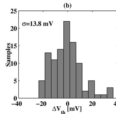
Fig. 4. Histogram distribution of 105 samples representing the threshold voltage variation caused by interface roughness. The results for (a) the [110] and (b) the [100] Si nanowire transistors are plotted.  $\sigma$  is the standard deviation of  $\Delta V_{\text{th}}$ .
