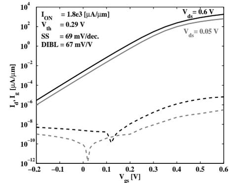
Fig. 5.  $I_d - V_{gs}$  and  $I_g - V_{gs}$  characteristics of a  $3 \times 3 \text{ nm}^2$  nanowire with TiN gates and stack layers of  $0.5 \text{ nm SiO}_2$  and  $3.25 \text{ nm HfO}_2$ .
