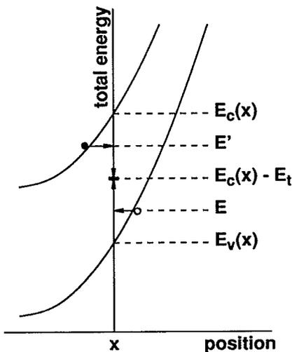
FIG. 1. One possible recombination path via a deep level at  $E_c(x) - E_t$  in a space-charge region.
