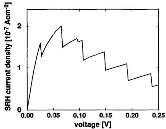
FIG. 7. SRH forward current density of a  $\delta$ -like trap configuration in the GaAs surface potential example of Fig. 4. The trap distance from the surface is 2 nm. Parameters:  $T = 300$  K,  $\tau_{n,0} = 10^{-15}$  s,  $\tau_{p,0} = 0$ ,  $U_{\text{bi}} = 0.85$  V, for other parameters see Fig. 4.
