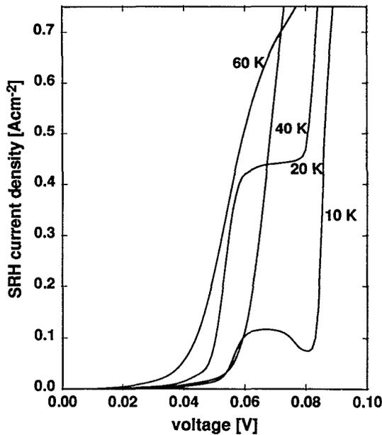
FIG. 6. SRH current density of the  $\text{Hg}_{0.8}\text{Cd}_{0.2}\text{Te}$   $n^+p$  diode of Fig. 5(a) for different temperatures: (1)  $T = 10$  K, (2)  $T = 20$  K, (3)  $T = 40$  K, (4)  $T = 60$  K. An acceptor binding energy of 6 meV and Fermi level pinning at the conduction-band edge in the  $n$  region have been assumed. For parameters see Fig. 5(a).
