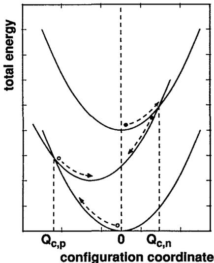
FIG. 2. Configuration-coordinate diagram with the crossing points of the harmonic potential parabolas at zero electric field. The two-band parabolas have to be replaced by a quasi-continuum of such parabolas, if the recombination takes place in an electric field. Then, both activation energies are lowered.
