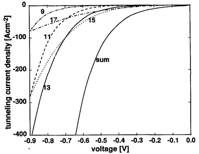
FIG. 4. Reverse bias tunneling characteristics of various  $n$ -phonon transitions ( $n$  indicated by the numbers) and the resulting sum. Parameters:  $T = 333$  K,  $S = 3.5$ ,  $\hbar\omega_0 = 33$  meV,  $\tau_{\text{eff}} = 10^{-6}$  s,  $E_g = 1.5$  eV,  $E_t = 0.75$  eV,  $m_c = 0.066m_0$ ,  $N_t = 10^{14}$  cm $^{-3}$ ,  $\epsilon_s = 12.9$ ,  $N_D = 10^{17}$  cm $^{-3}$ ,  $U_{bi} = 0.45$  eV.
