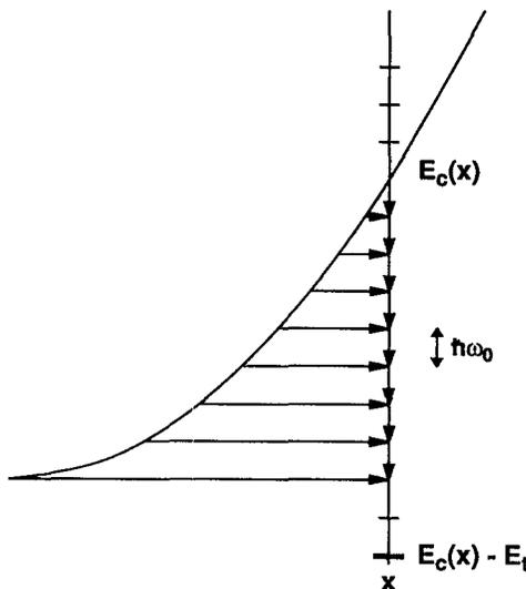
FIG. 3. Electron recombination paths: tunneling to the trap and subsequent thermal capture.
