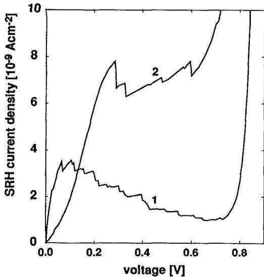
FIG. 8. SRH forward current density of the GaAs surface potential of Fig. 7 with uniformly distributed traps on a grid with (1)  $\Delta x_i = d = 0.565 \text{ nm}$ ,  $N_D = 5 \times 10^{17} \text{ cm}^{-3}$  and (2)  $\Delta x_i = 2d$ ,  $N_D = 1 \times 10^{17} \text{ cm}^{-3}$ . Parameters:  $\tau_{n,0} = \tau_{p,0} = 10^{-15} \text{ s}$ , other parameters unchanged.
